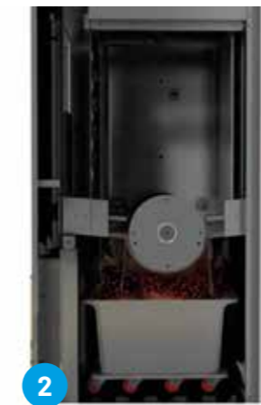
2 The waste gets shredded and vacuum is applied to remove cold spots of entrapped air.
