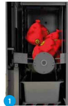
1 The waste is introduced by gravity inside the chamber from the top.
